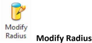
Use this command to modify the radius of cylinder and sphere.
