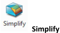
Use this command to simplify a part by removing selected faces. The command will attempt to extend and reconnect faces to close the resulting gaps in the part. If the part cannot be closed properly an error message will be returned. Select the faces to remove and then middle-click to remove them.
